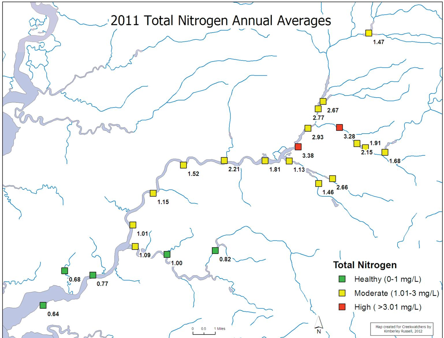
TN generally improved in the downstream direction, indicating high N sources upstream and dilution with lower N tidal waters coming from Tangier Sound. Water clarity was consistently poor, with Secchi depth at all but one station below the threshold of 36 inches (91.4 cm). This is likely influenced by the shallow, well-mixed nature of this system, which may result in higher
